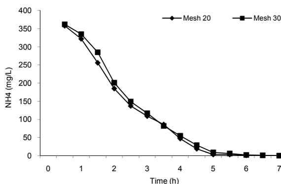
Fig. 3: Ammonium elution by regenerant solution (1M CINa) in column system
