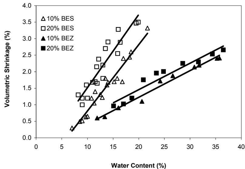
**Figure 11.** Comparison of volumetric shrinkage of BES (open signs) with those of BEZ (filled signs), (BES data from Kraus et al., 1997). Lines on the data show the linear regression lines.
