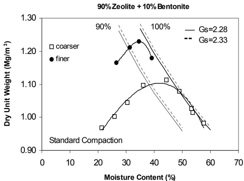
**Figure 10.** The effect of grain size on the compaction characteristics of BEZ.
