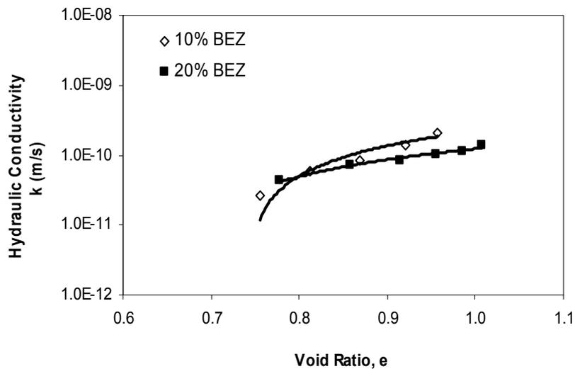
**Figure 5.** Hydraulic conductivity of BEZ with 10% and 20% bentonite as a function of void ratio.
