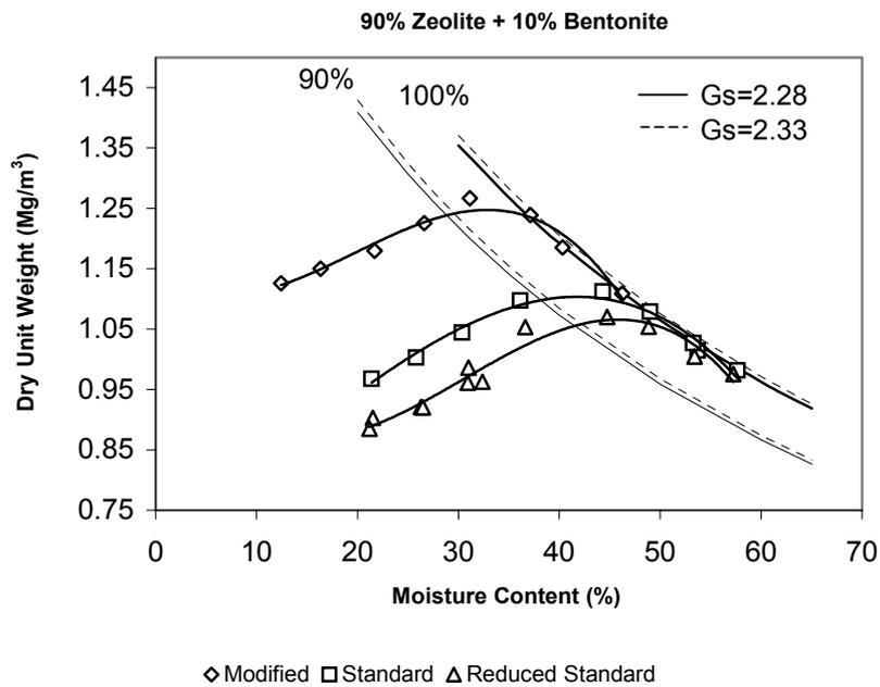
**Figure 9.** The effect of compaction energy of BEZ with 10% bentonite and 90% Gordes zeolite. The effect of the grain size is shown in Figure 10.
