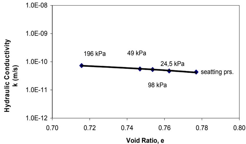
**Figure 6.** Variation of hydraulic conductivity with respect to void ratio of 20% BEZ samples for different initial seating pressures (after Kaya and Durukan, 2004)
