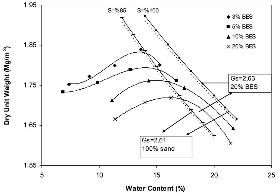
**Figure 8.** Compaction characteristics of bentonite embedded sand with various bentonite contents.
