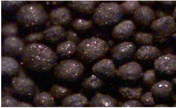
Fig. 4. Zeocarbon type microcapsules viewed by optical microscope (290–680 \mu\text{m} ).
