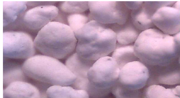
Fig. 3. Zeolite type microcapsules viewed by optical microscope (500–1000 μm).
