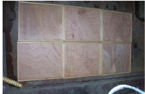
(b) specimen set with wooden formworks
