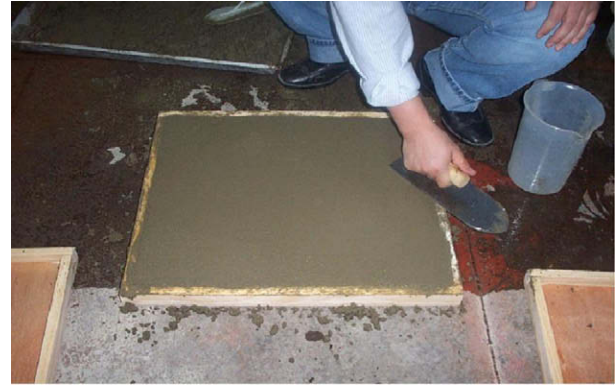
(a) mortar panel specimen containing microcapsules
